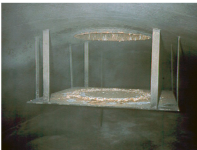
(c) Example of an inlet impingement plate.
